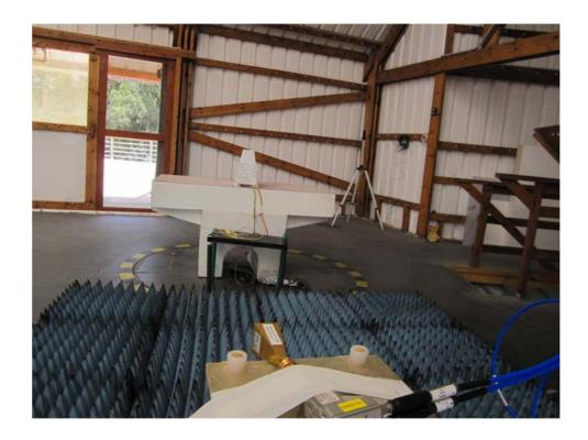
Photograph No.6 Spurious emissions measurement setup at the OATS above 40 GHz
