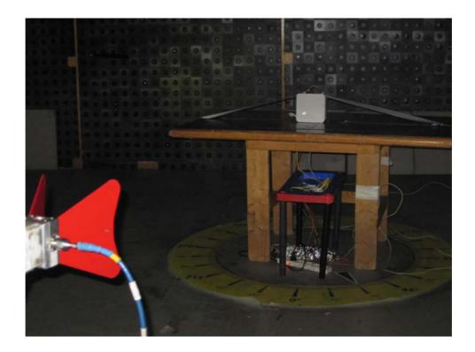
Photograph No.5 Spurious emissions measurement setup at the OATS in 18-40 GHz
