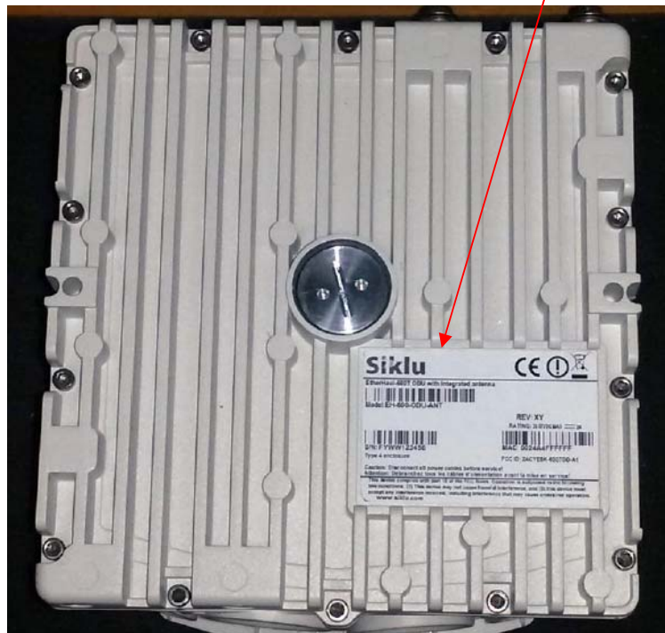
EtherHaul EH-600T top panel, label with FCC ID:2ACYESK-60GTDD-A1 location
