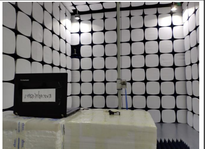
Radiated Spurious Emissions Test Setup Above 1GHz
