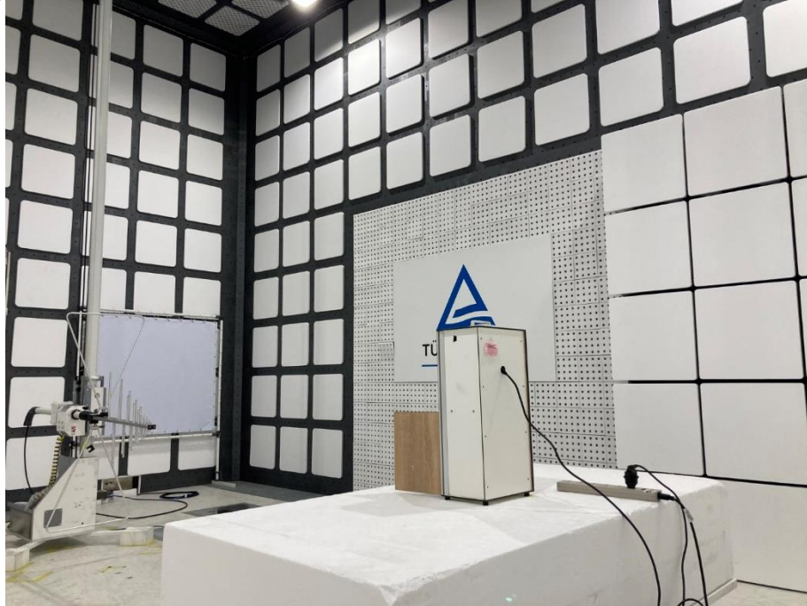
Photograph 3: Test Setup for Spurious Emissions (Back View 2)
