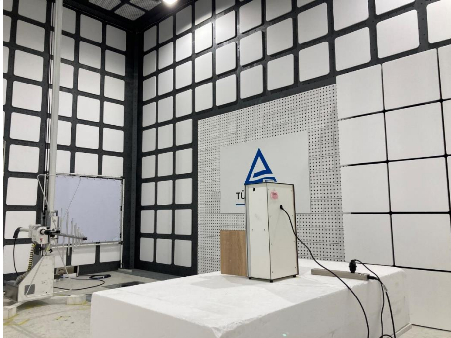
Photograph 8: Test Setup for Spurious Emissions (Back View 2)
