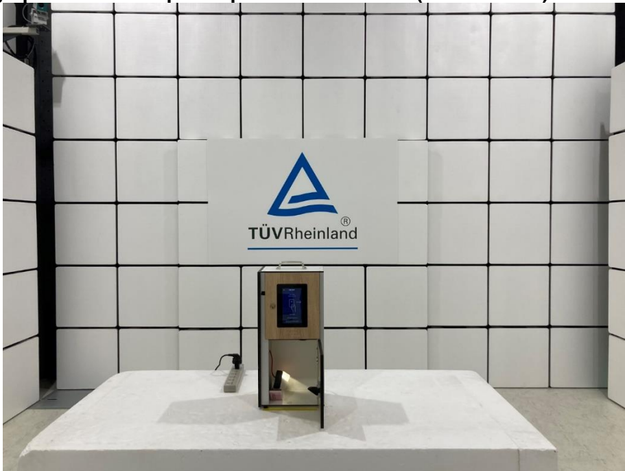
Photograph 6: Test Setup for Spurious Emissions (Front View 1)
