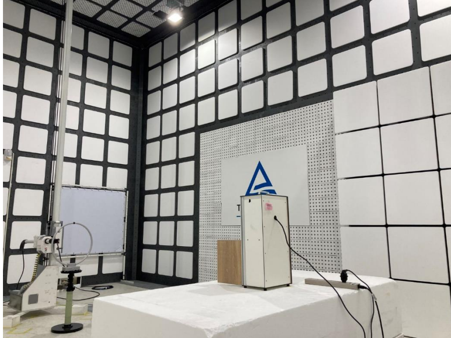
Photograph 7: Test Setup for Spurious Emissions (Back View 1)
