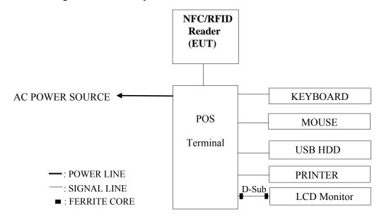
No. 1 10m Semi-Anechoic Chamber Setup Diagram (Test distance:10m) for 30-1000MHz 5.2.2.
