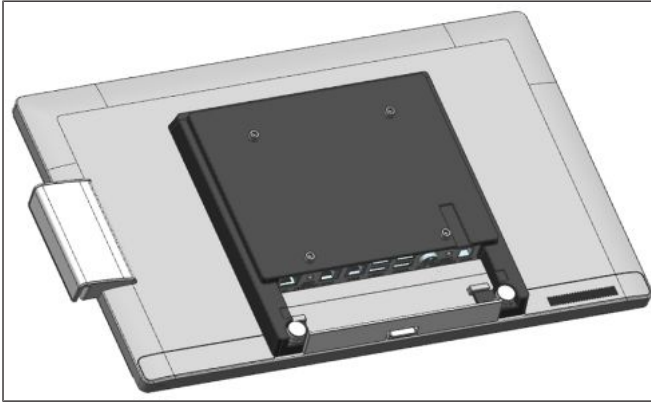
Figure 14-15: MSR module installed
