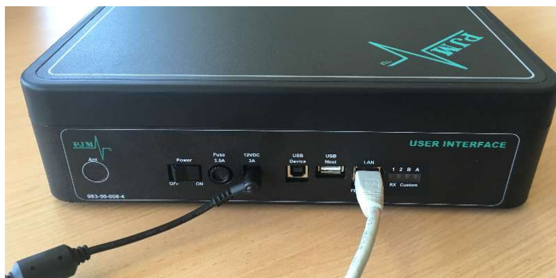
MDR-4330AT with power & Ethernet cables connected
