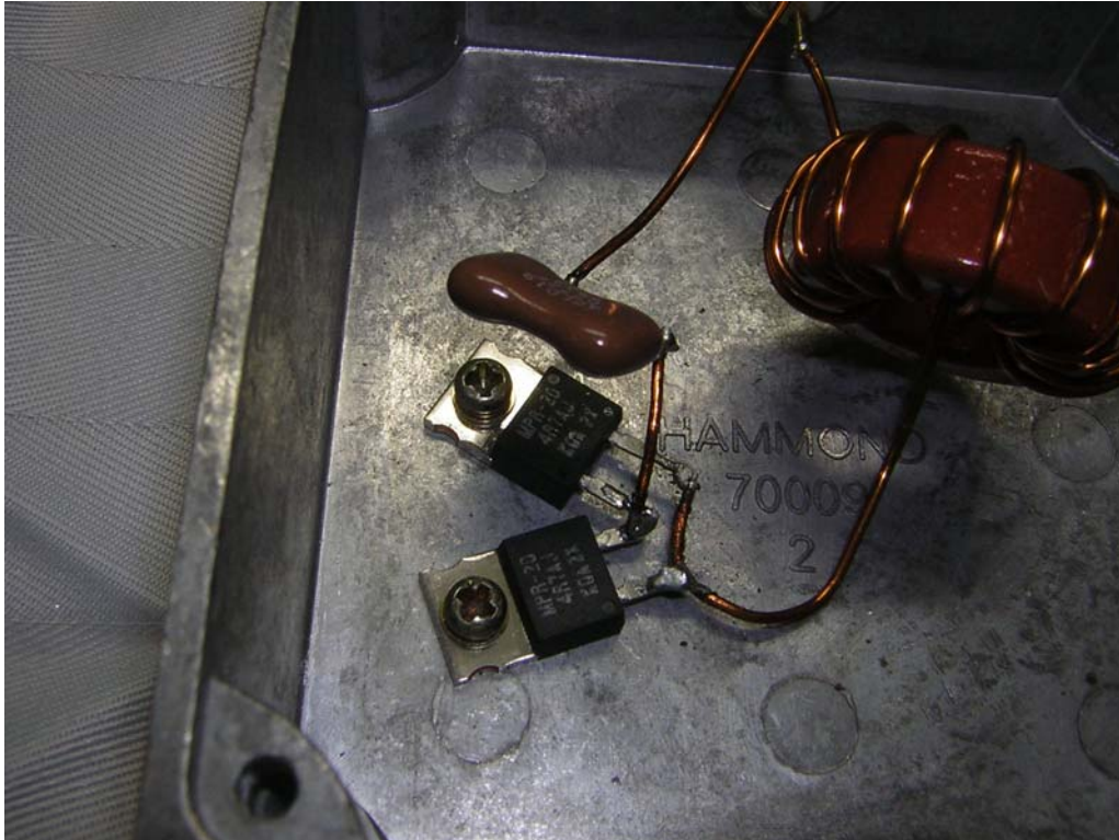
Internal of 50Ω Termination Box
