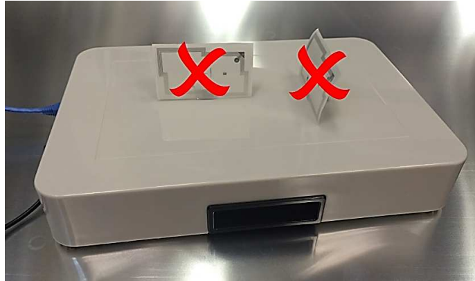
Incorrect Tag Orientation
