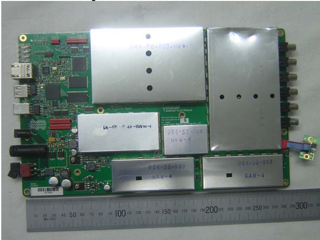
EUT PCB with Shielding
