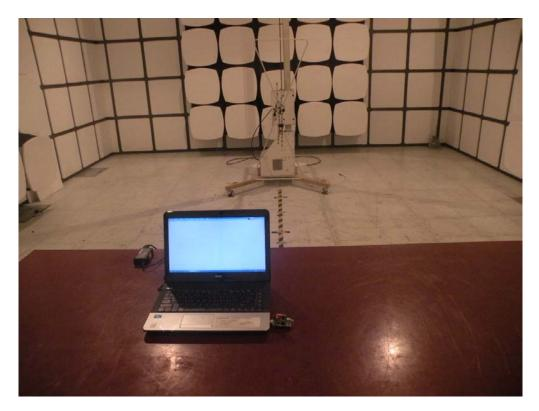
Radiated Emission Test Setup in Chamber
