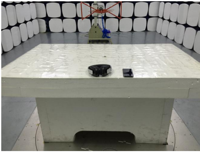
Radiated Spurious Emissions Test Setup Below 1GHz
