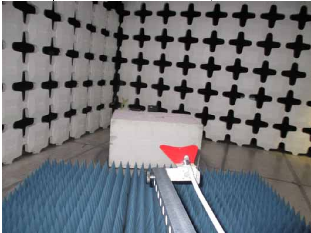
Test Setup for Radiated Emissions – 1GHz to 2.5GHz, Vertical Polarization
