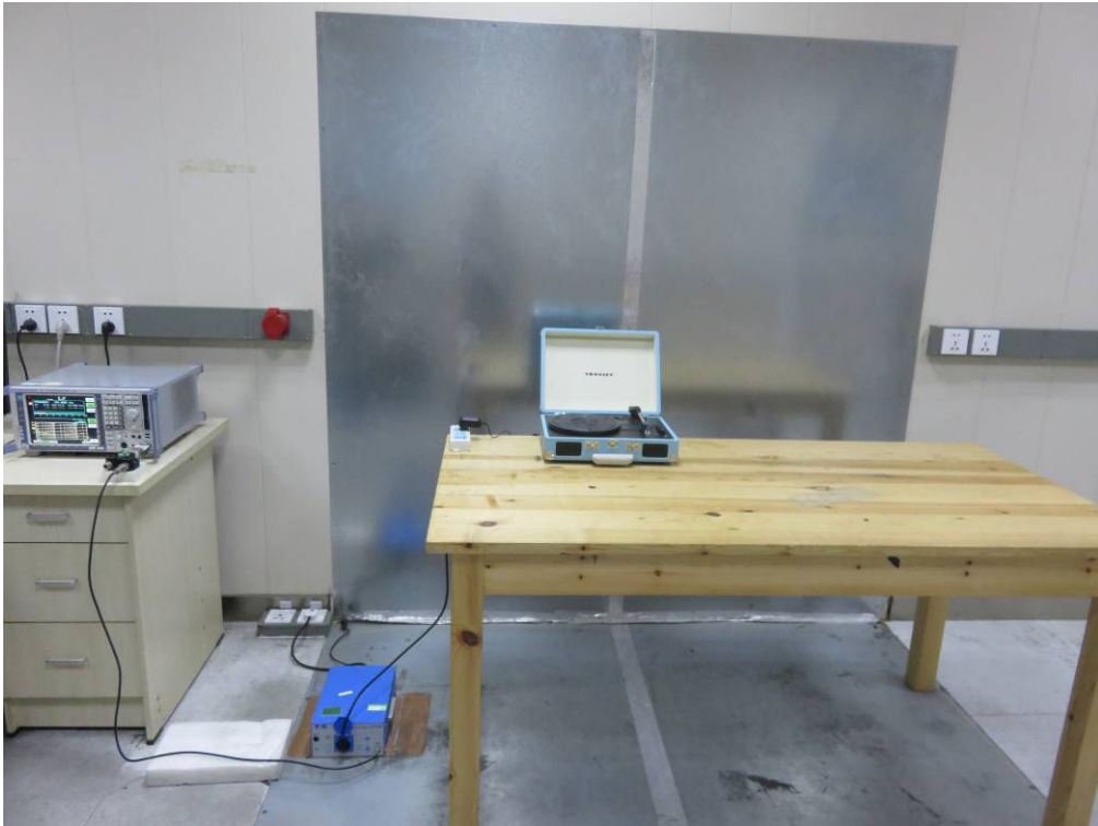
FCC LINE CONDUCTED EMISSION TEST SETUP-2
