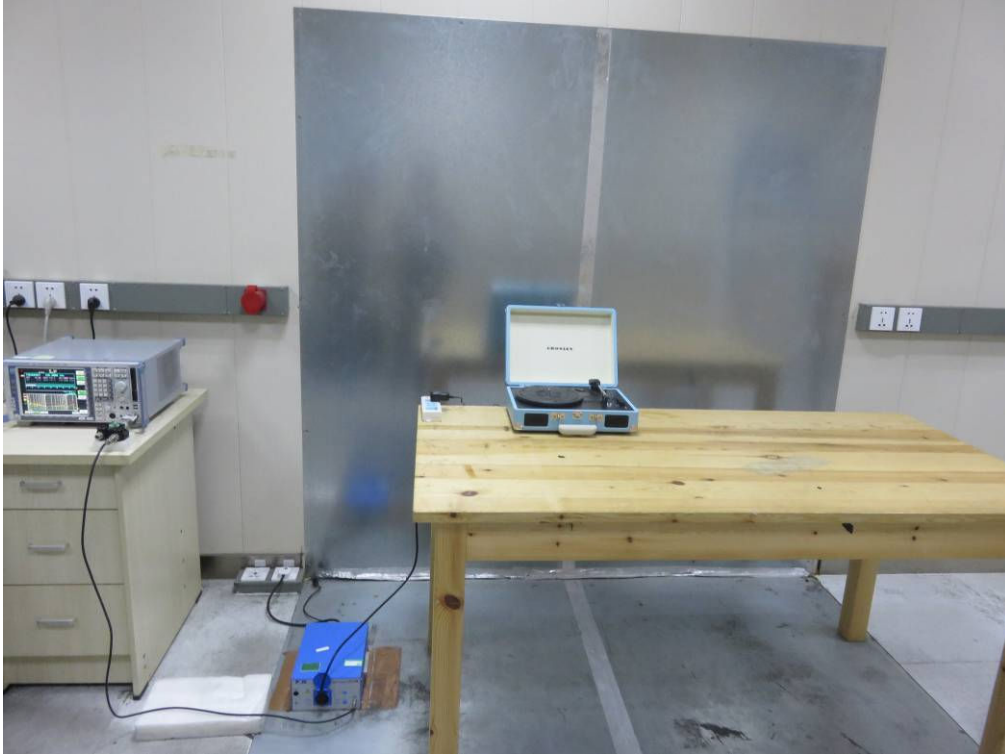
FCC LINE CONDUCTED EMISSION TEST SETUP-2
