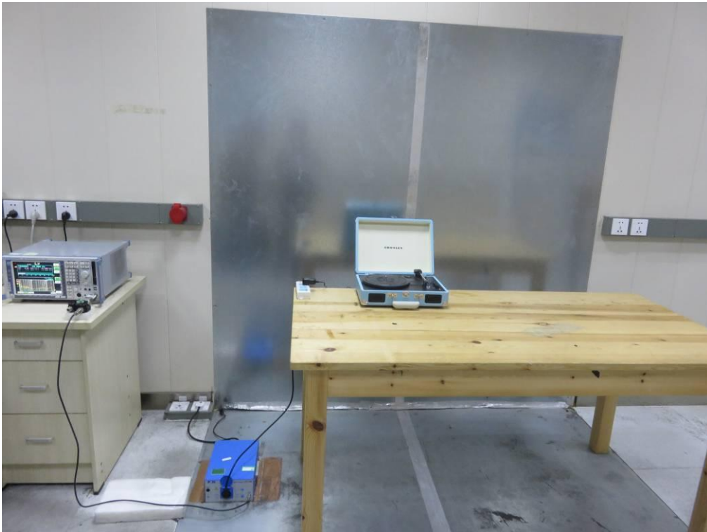
FCC LINE CONDUCTED EMISSION TEST SETUP-2
