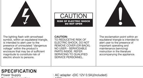
Power Supply Power Consumption Speed Speaker Replacement Needle : AC adapter -(DC 12V 0.5A)(Included) : 12W : 33<sup>1</sup>/<sub>3</sub> / 45 /78 RPM : 8Ω /5W x 2 : NP-6
