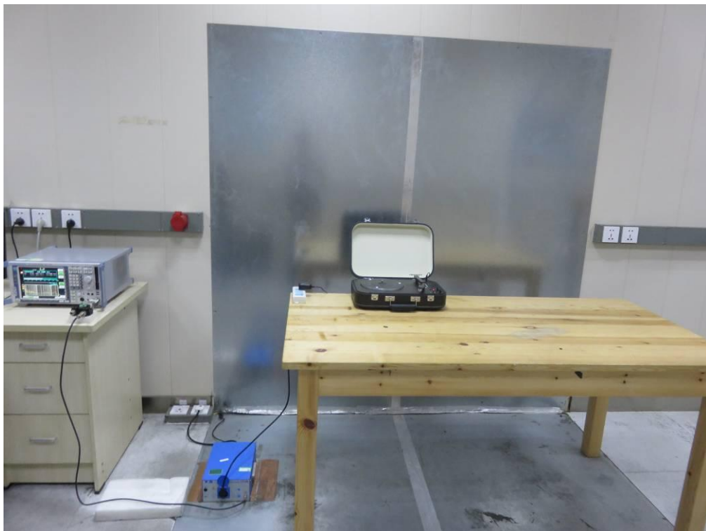
FCC LINE CONDUCTED EMISSION TEST SETUP-2
