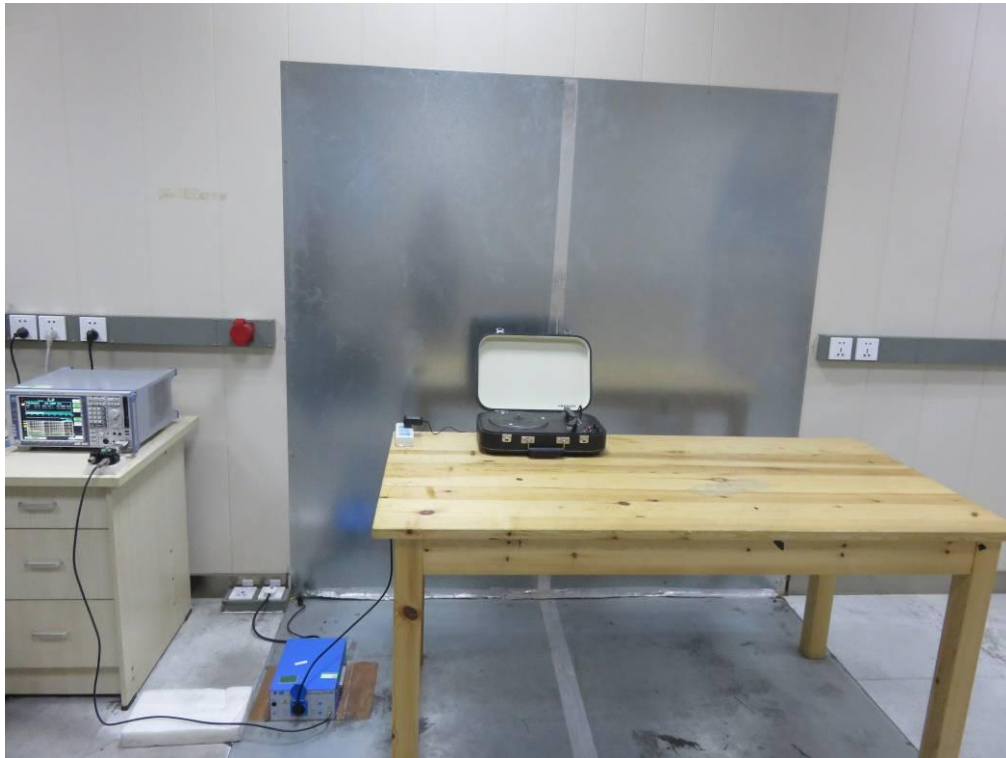
FCC LINE CONDUCTED EMISSION TEST SETUP-2
