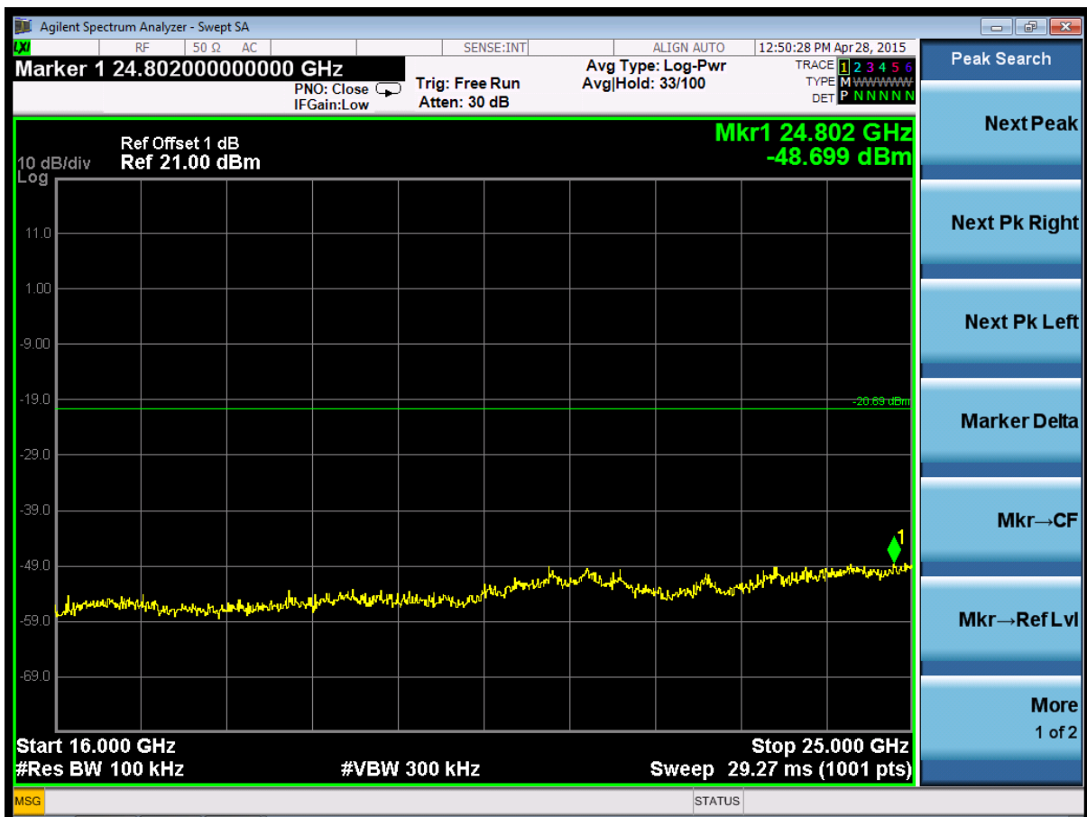
(Plot 4.7.2 C6: Channel 11: 2462MHz @ 802.11g)
