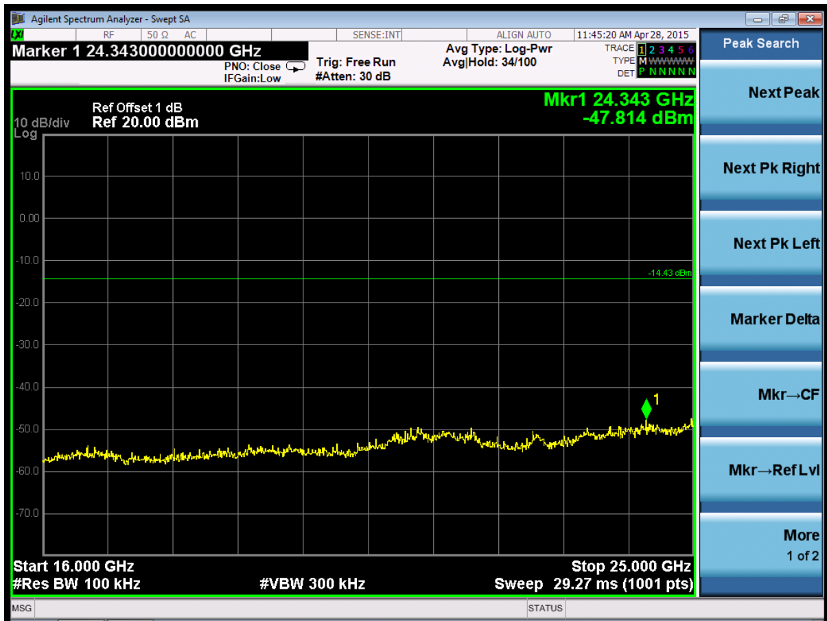
(Plot 4.7.1 C5: Channel 11: 2462MHz @ 802.11b)
