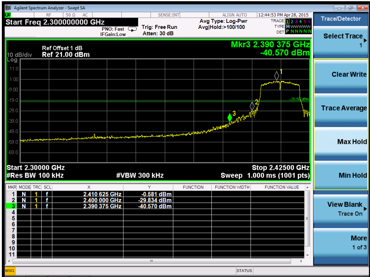
(Plot 4.7.2 D: Channel 1: 2412MHz @ 802.11g)
