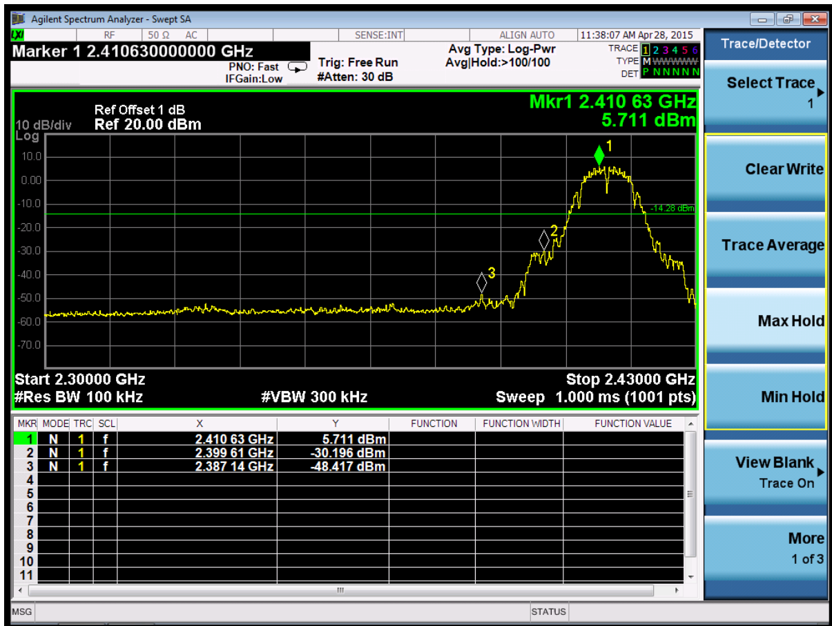
(Plot 4.7.1 D: Channel 1: 2412MHz @ 802.11b)
