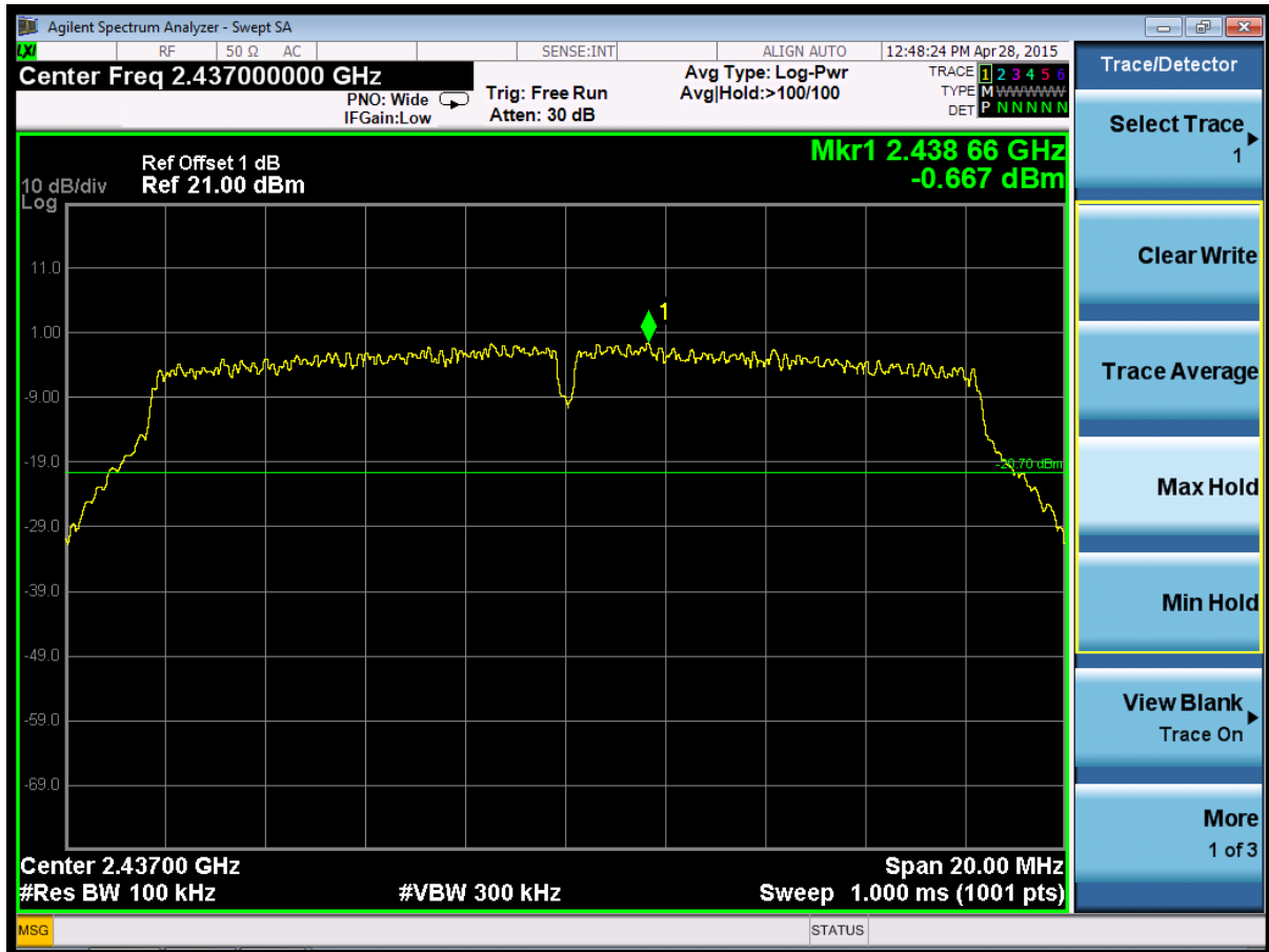
(Plot 4.7.2 B1: Channel 6: 2437MHz @ 802.11g)
