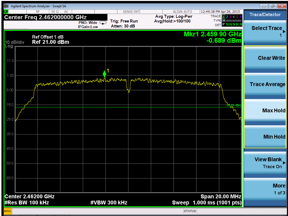
(Plot 4.7.2 C1: Channel 11: 2462MHz @ 802.11g)
