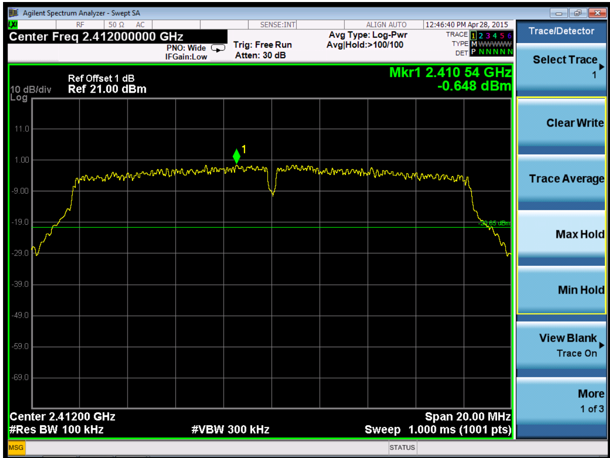
(Plot 4.7.2 A1: Channel 1: 2412MHz @ 802.11g)
