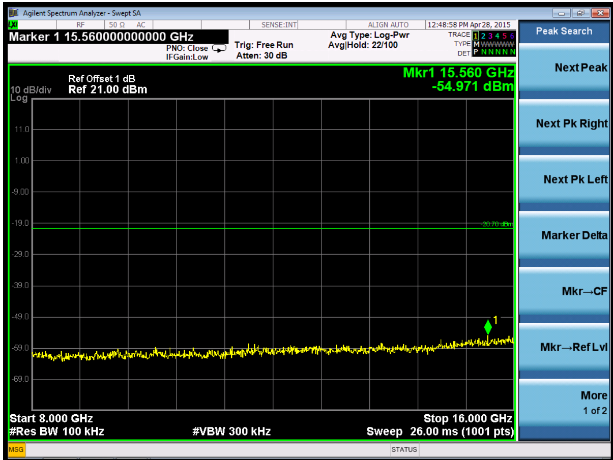
(Plot 4.7.2 B5: Channel 6: 2437MHz @ 802.11g)
