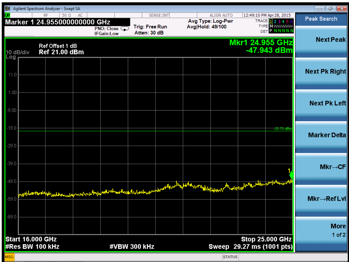
(Plot 4.7.2 B6: Channel 6: 2437MHz @ 802.11g)
