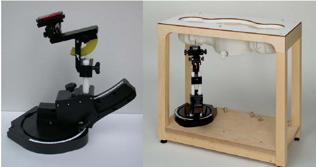
Device holder supplied by SPEAG
