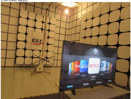
Radiated Test (1000-25000 MHz)
