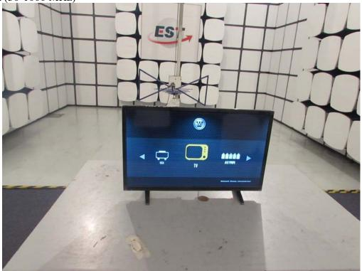
Radiated Test (1000-25000 MHz)
