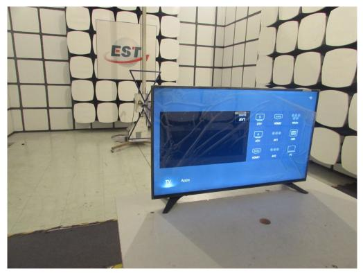
Radiated Test (1000-25000 MHz)
