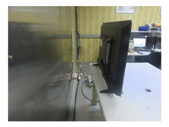
Radiated Test (30-1000 MHz)
