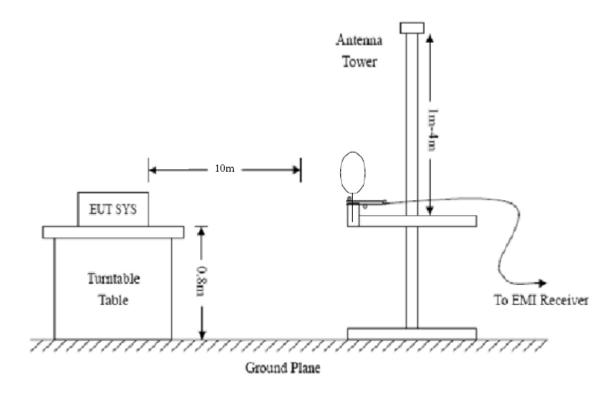
Frequency:9kHz-30MHz Frequency:30MHz-1GHz Frequency: Above 1GHz RBW=10KHz, RBW=120KHz, RBW=1MHz, VBW = 30KHzVBW=300KHz VBW=3MHz(Peak), 10Hz(AV) Sweep time= Auto Sweep time= Auto Sweep time= Auto Trace = max holdTrace = max holdTrace = max holdDetector function = peak Detector function = peak, QP Detector function = peak, AV
