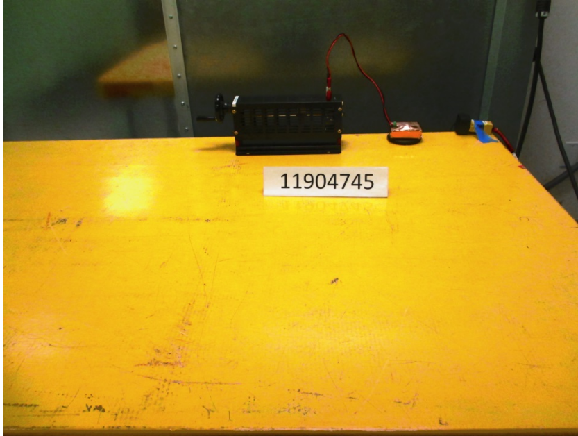
FRONT- WITH 15W LOAD (RX SIMULATOR SHIELDED WITH COPPER TAPE)
