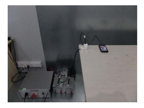
Radiation Emission Test Setup (Below 30MHz)
