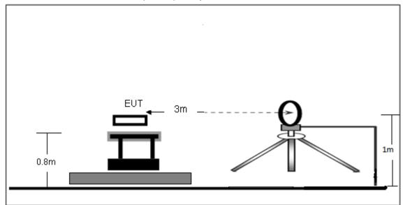
(B) Radiated Emission Test-Up Frequency 30MHz~1GHz
