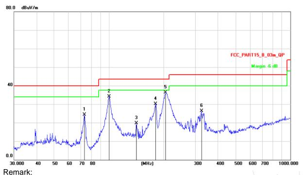
Factor = Antenna Factor + Cable Loss – Pre-amplifier.
