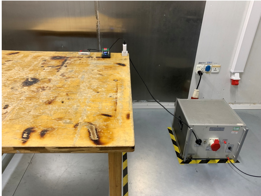
Photograph – Conducted Emission Test Setup
