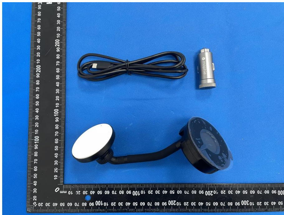
EUT Photo 1 (wireless charging window & dash mount with Magsafe)
