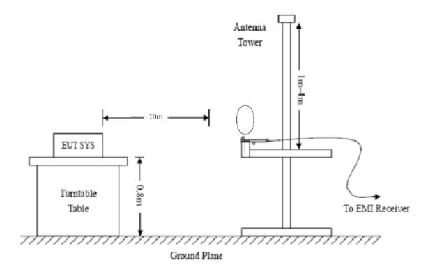
Frequency:9kHz-30MHz Frequency:30MHz-1GHz Frequency: Above 1GHz RBW=10KHz, RBW=120KHz, RBW=1MHz, VBW=300KHz VBW = 30KHzVBW=3MHz(Peak), 10Hz(AV) Sweep time= Auto Sweep time= Auto Sweep time= Auto Trace = max holdTrace = max holdTrace = max holdDetector function = peak Detector function = peak, QP Detector function = peak, AV
