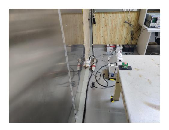
Radiated Test (9kHz-30 MHz)
