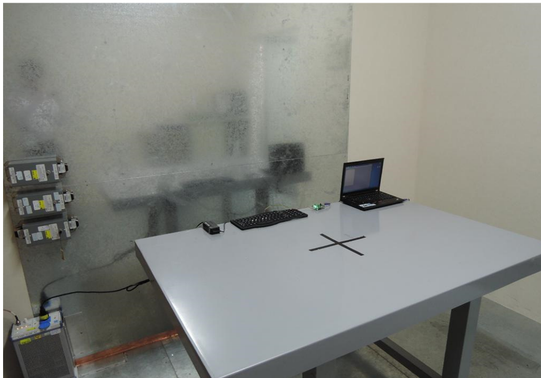
Photograph 6: Set-up for for Mains Conducted testing Front
