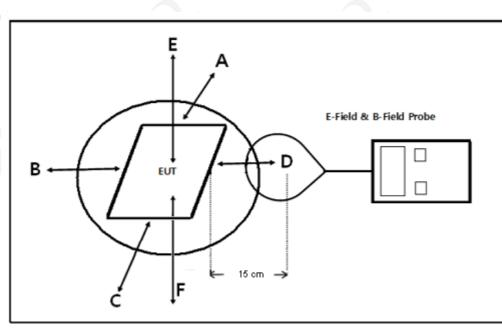
Note: Due to installation limitations no tests from the underside of the charging device (Test Position F) are required.
