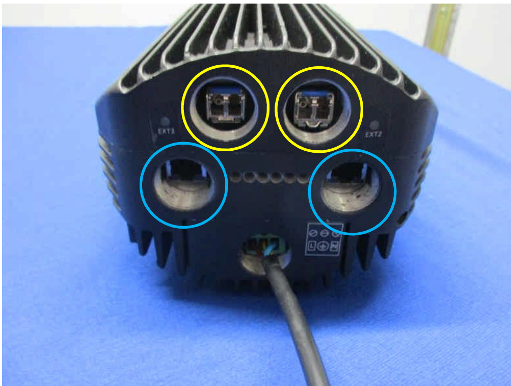
Photograph shows the optical fibre ports (highlighted yellow) and Ethernet ports (highlighted blue)
