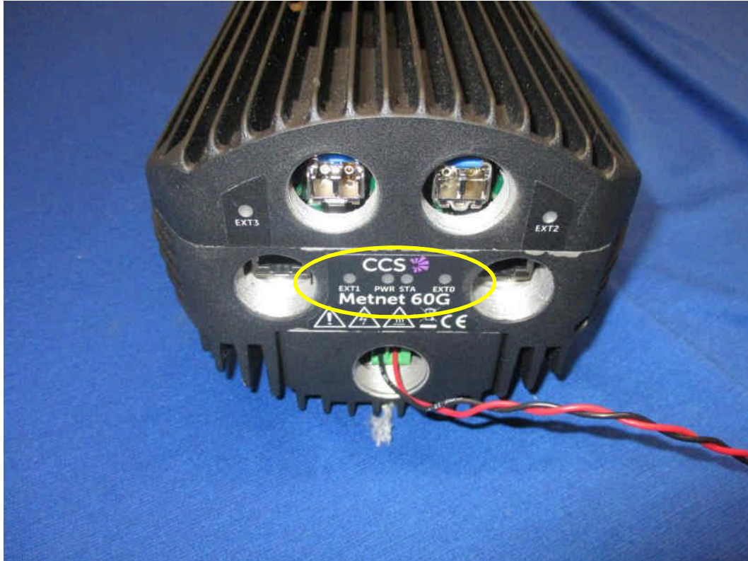
Photograph shows the EUT's status LED's (highlighted)
