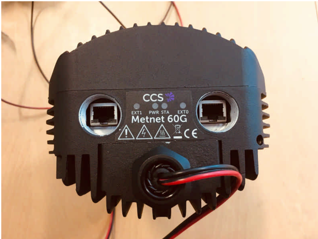
c) PoE/48V powered without fibre
