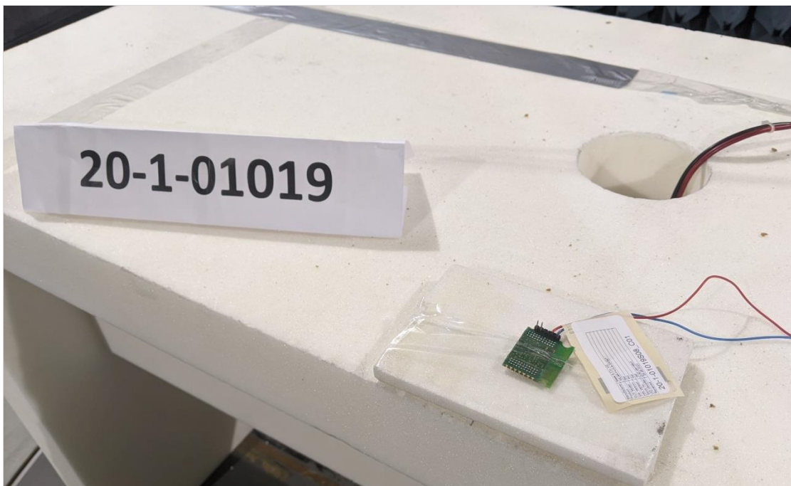
Photograph 2: EUT Test Setup in the semi anechoic chamber, Radiated interference field strength
