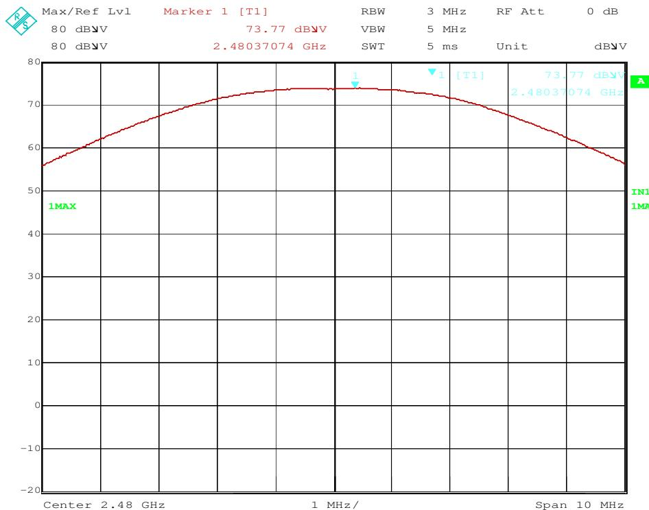
The highest antenna gain is 2.0 dBi. Therefore no reduction of the Peak power limit is necessary.
