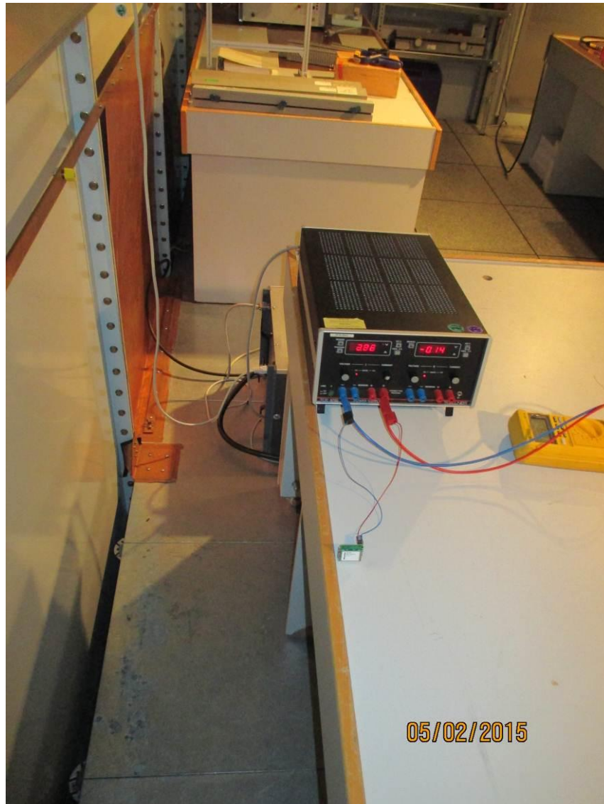
150729_22: Test setup – conducted emissions on power supply lines
