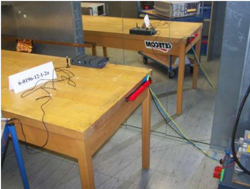
EMI AC – Power lines conducted test with power supply 110 AC V/ 60 Hz, EUT C
