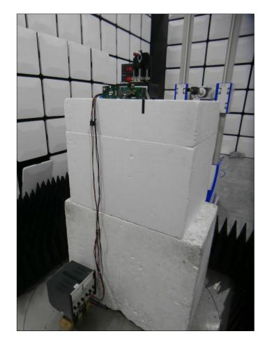
Figure 3 - Test Setup - 18 GHz to 25 GHz
