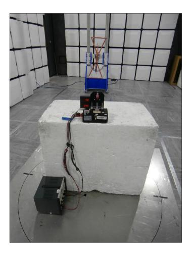
Figure 1 - Test Setup - 30 MHz to 1 GHz
