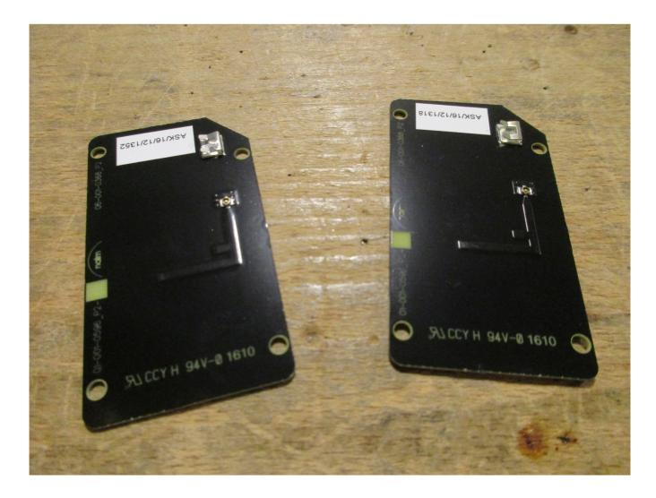
Description: Alternative antennas not used for measurements (lower gain)
