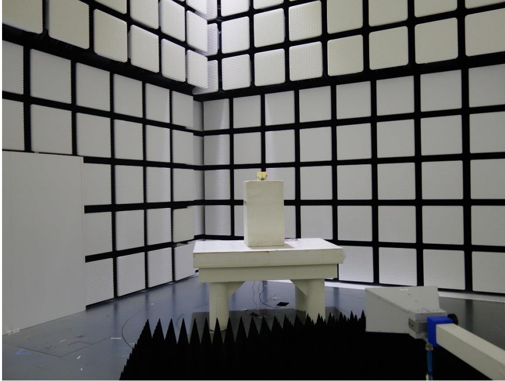
Photograph 5: Set-up for Radiated Emission above 1GHz, Front View
