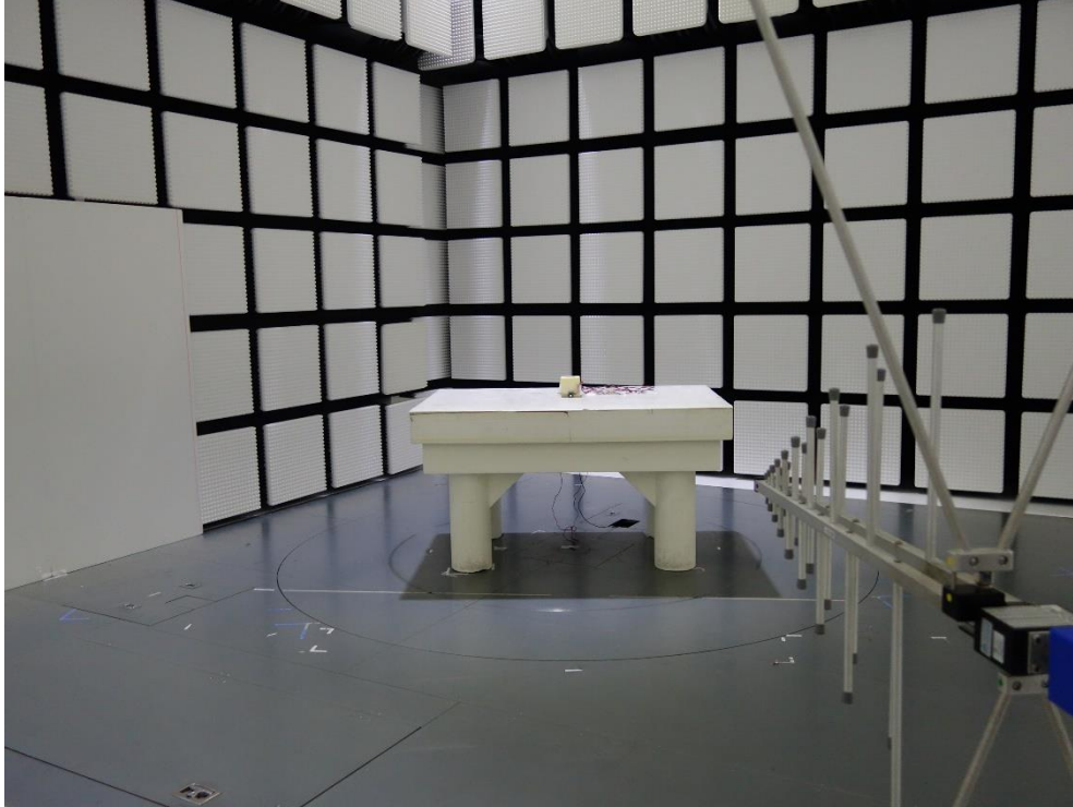
Photograph 3: Set-up for Radiated Emission below 1GHz, Front View
