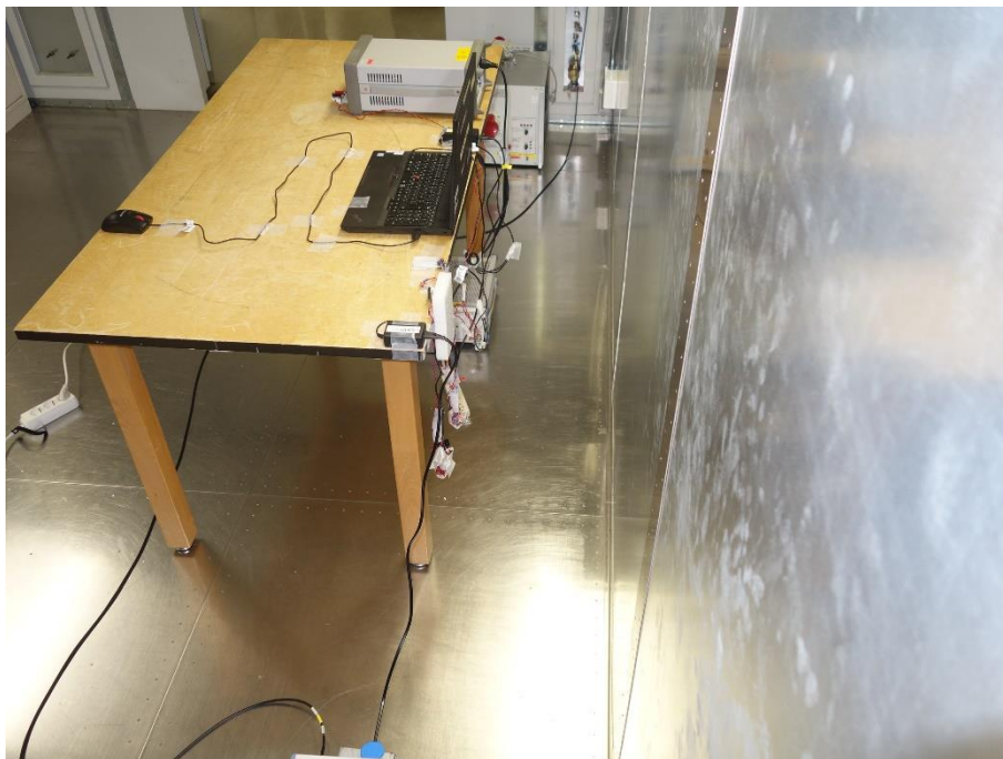
Photograph 2: Set-up for AC Power Line Conducted Emission, Rear View
