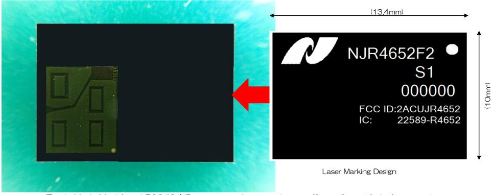
Trade Mark, Model and FCC/ICs' ID are wrote direct on the surefface of module by laser marking. Life time: over 10years
