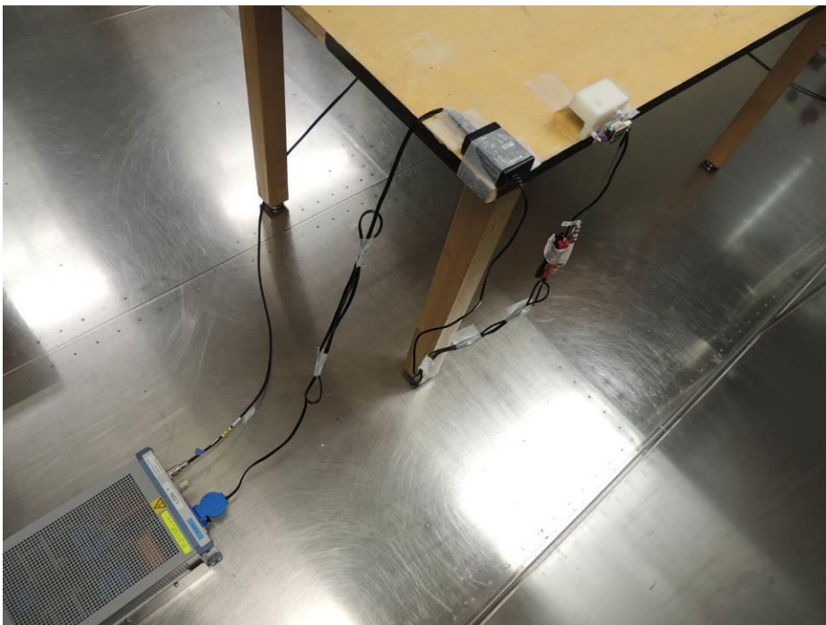
Photograph 2: Set-up for AC Power Line Conducted Emission of Transmitter, Rear View
