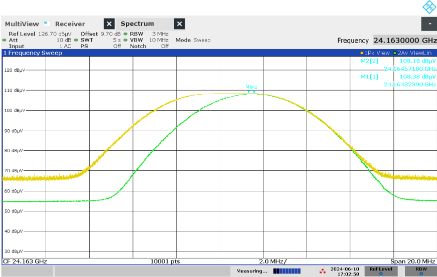
Figure 5: Field Strength of Fundamental, Spectral Diagram, Mode C
