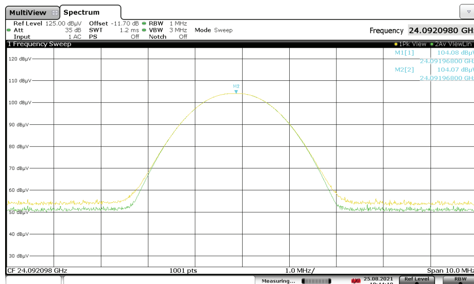
Figure 9: Field Strength of Fundamental, Spectral Diagram, Configuration 1, DC 5V
