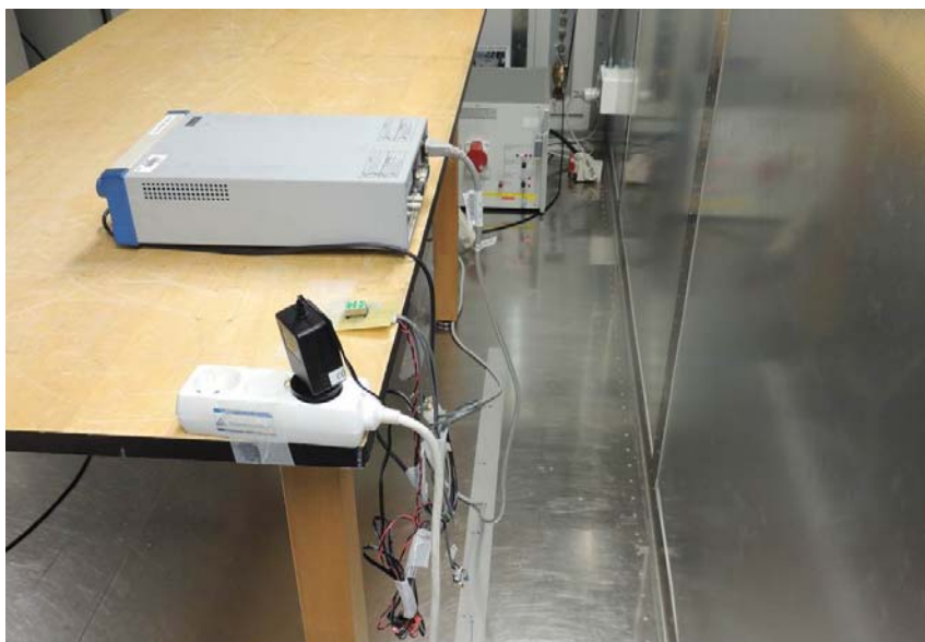
Photograph 2: Set-up for AC Power Line Conducted Emission of Transmitter, Rear View
