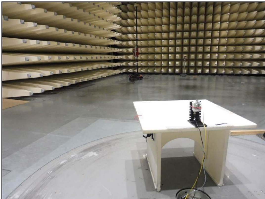
Photo 2: radiated emission 30MHz - 1GHz set 1
