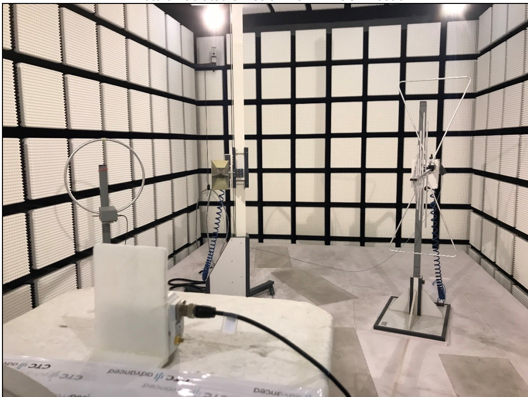
Photo 6: radiated emission 1GHz - 18GHz set 3
