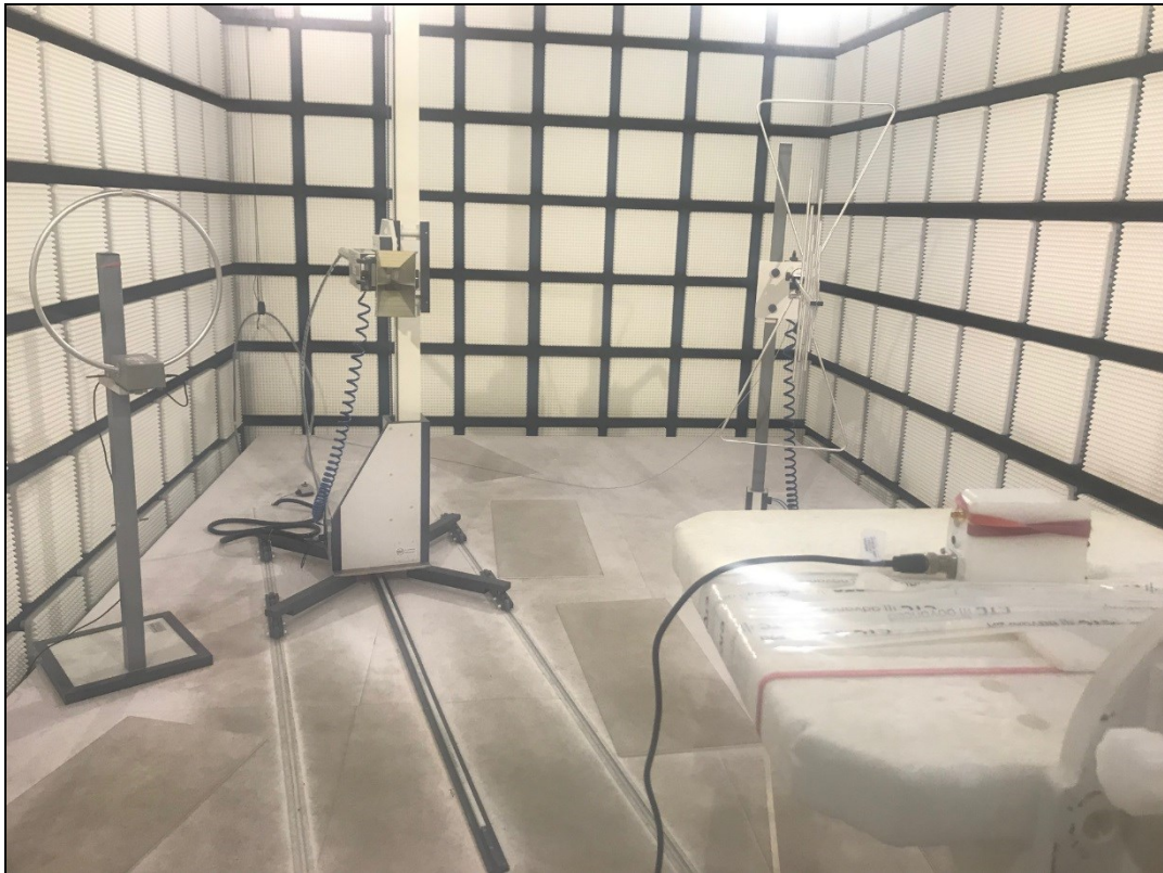
Photo 3: radiated emission 1GHz - 18GHz set 1
