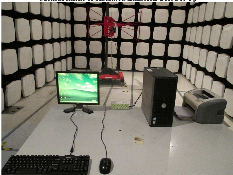
Measurement of Radiated Emission Test Set Up
