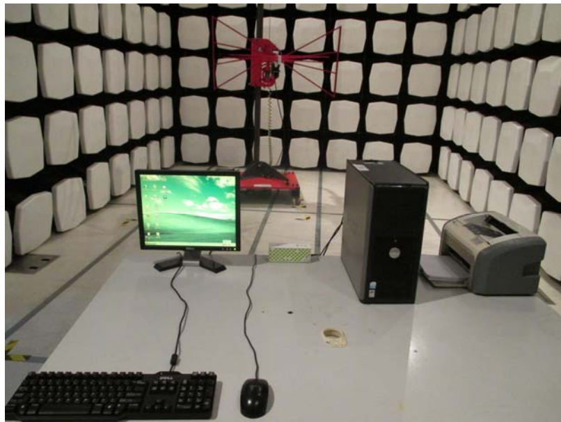
Measurement of Radiated Emission Test Set Up
